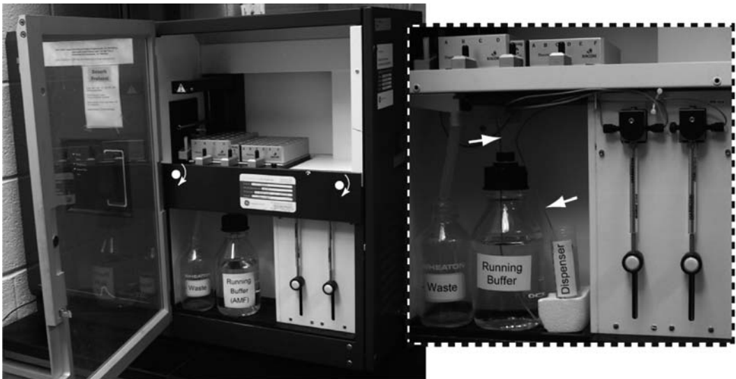
Fig. 5.1. Identification of left and right pump inlets on Biacore 3000. Loosen the two screws ( white circles/arrows ) on the panel to remove the cover. This allows the user to trace each inlet back to the right and left pump. The Biacore Running Buffer should be placed in the inlet corresponding to the left pump while the right pumps inlet should be submerged in Dispenser Buffer.
